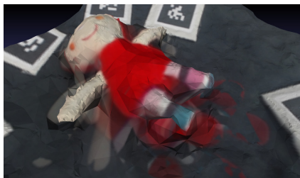
Figure: Reconstruction with the open-source state-of-the-art MVS pipeline AliceVision [AliceVision, 2017] with 4 images (right)
