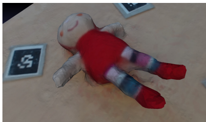
Figure: Reconstruction with the open-source state-of-the-art MVS pipeline AliceVision [AliceVision, 2017] with 30 images (right)
